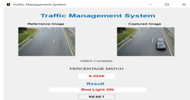
Figure 5(b) Image Matching Result causing light to turn "RED".
