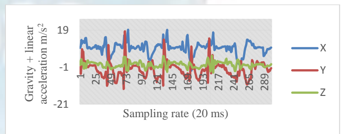
Figure 6: Raw data of the smartwatch accelerometer sensor for walking down stair activity
