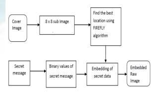
Fig 1. Data hiding using Firefly algorithm
