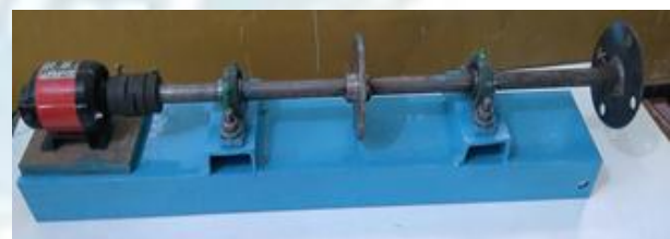
Fig: TEST SETUP FOR VIBRATION ANALYSIS
