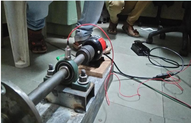
MOUNTING POSITION AT BEARING 1
