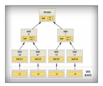
Figure 1: Block Hash Tree Structure
