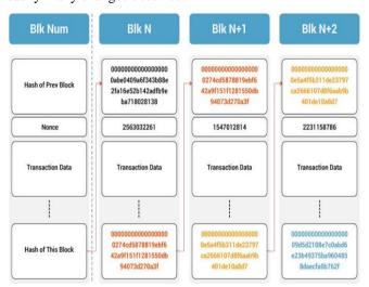
Figure 2: Block Hash Calculations
