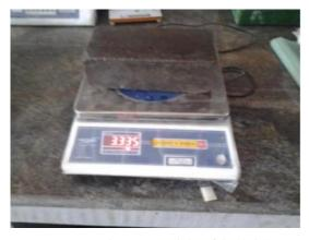
Figure 6. Weight of dry brick
