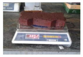
Figure 7. Weight of wet brick
