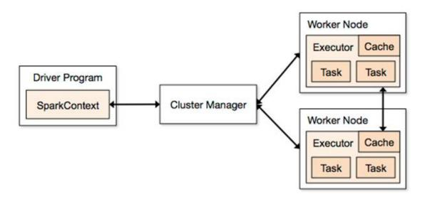
Fig 2. Architecture of Spark
