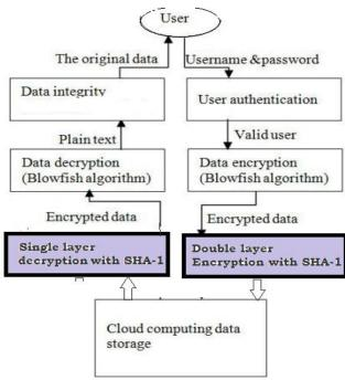
Fig 4. Data encryption and Decryption using symmetric algorithms
