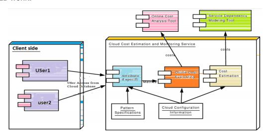
Fig 1.Cloud Cost estimation and Monitoring Service Model
