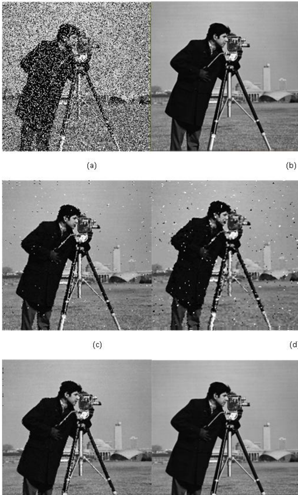
Fig 1.a) Cameraman image corrupted with 30% noise density, (b) Output of PA, (c) Output of DBA, (d) Output of MF, (e) Output of MDBUTMF, (f) Original Image
