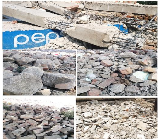
Figure 2: Demolished wastes of structural elements
