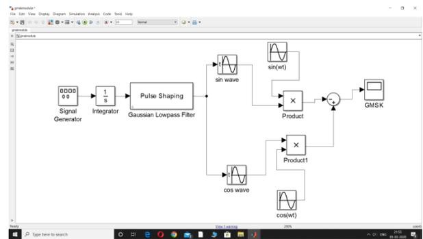
Fig 5.7: Simulation of GMSK Modulation.
