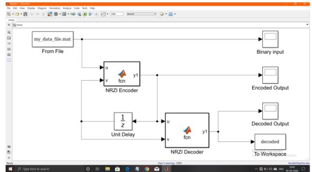
Fig 5.2 Simulation of encoder and decoder
