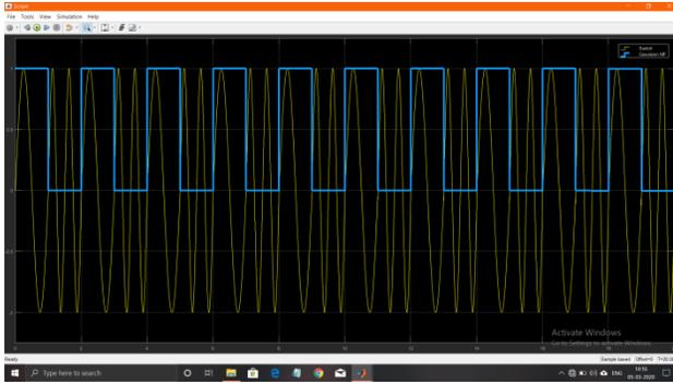
Fig 5.8 Output of GMSK Modulation
