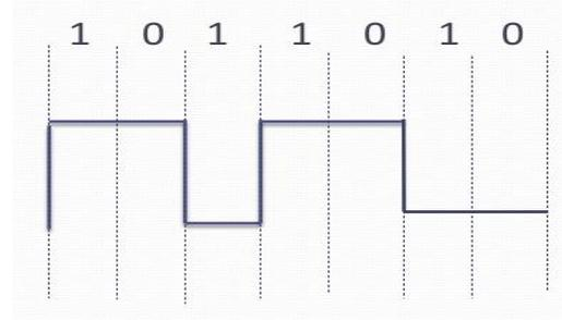
Fig 5.1 NRZI Encoding
