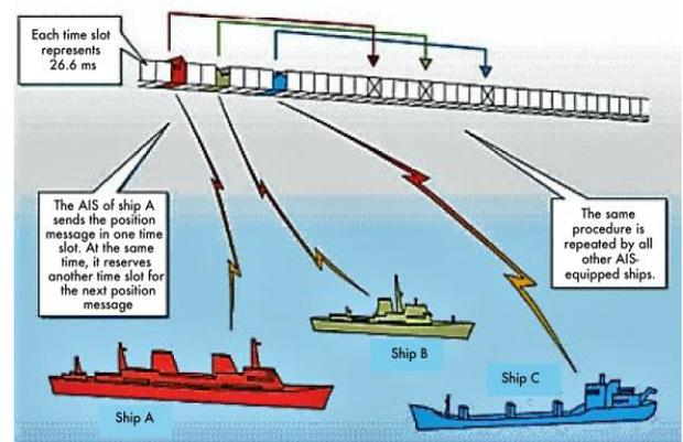
Fig 1: AIS messages transmission by Ship Transponders and slot assignment
