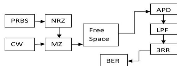
Figure 5.1 System Model of FSO Communication
