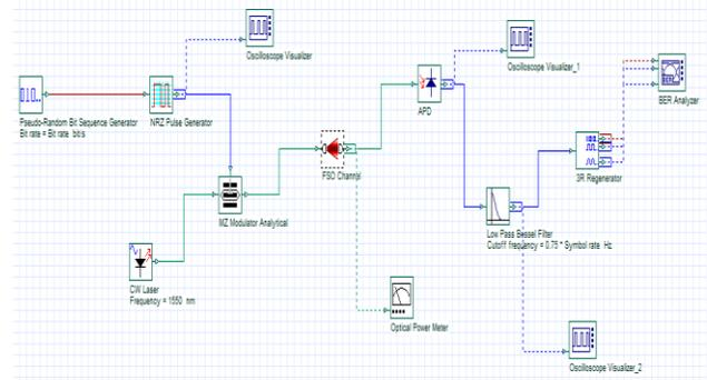
Figure 5.2 Optimized 1550 nm FSO Link Design
