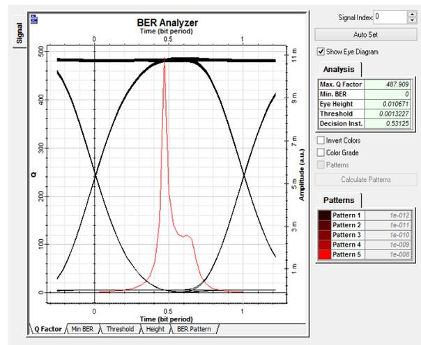
Figure 6.1 Simulation Result for Clear Sky at 0.5 km
