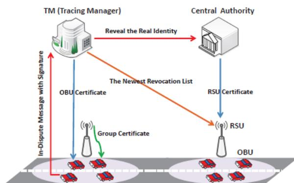
Our architecture demonstrates made out of the accompanying gatherings: the focal specialist (CA), the following tracer (TM), many RSUs, and numerous OBUs, as appeared in Fig. The CA is in charge of confirming general society keys of RSUs. After confirmation, the CA will issue the key certificates. The TM is responsible for confirming the public keys of OBUs. After validation, the TM will issue the key certificates. The TM is likewise ready to give the sender the identity who communicates a
