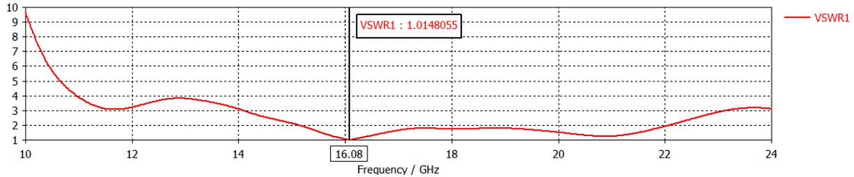
Fig 2(e) VSWR of proposed antenna design
