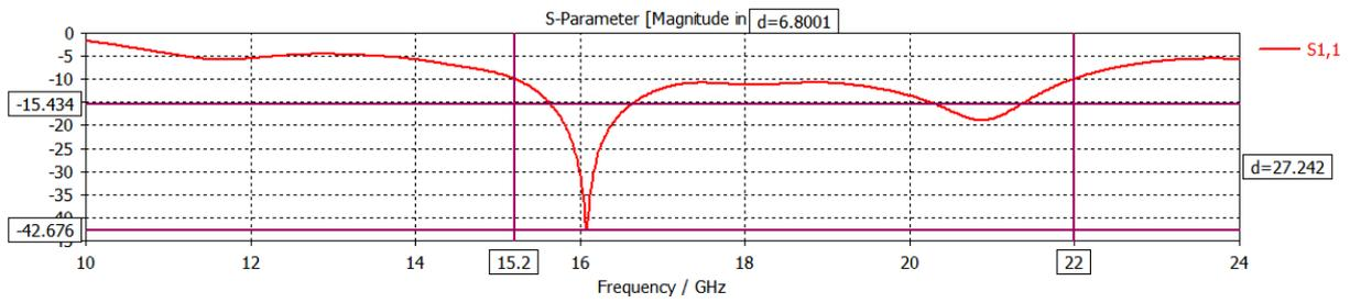
Fig. 2(a) Return loss (S11) plot of the proposed antenna design
