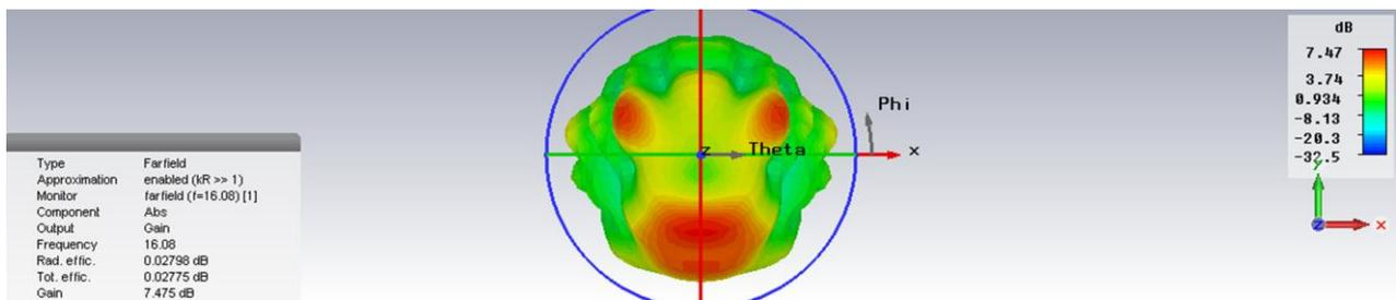
Fig. 2(b) Gain of proposed antenna design
