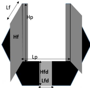
Fig.1 (c) Top view of the proposed antenna design
