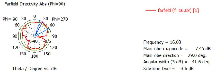
Fig 2(d) HPBW plot of proposed antenna design
