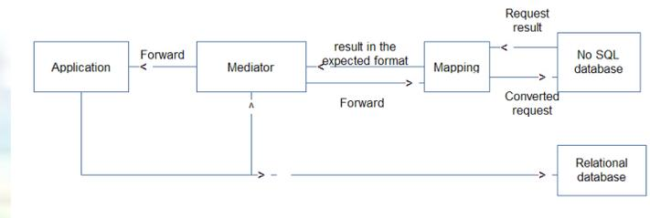
Figure 2: Data Mapping Module Working Diagram
