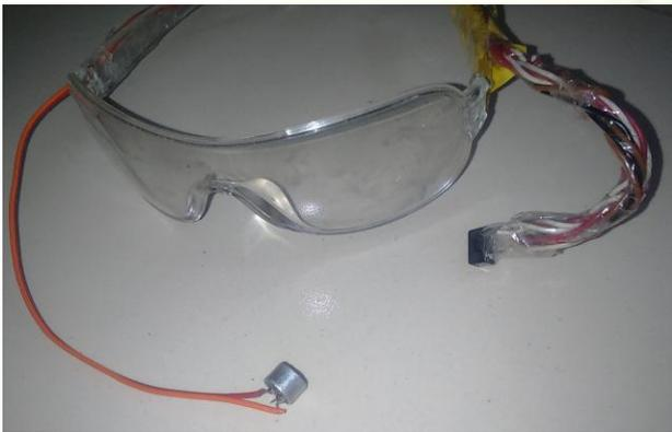
Fig.6. MIC and Reflection Sensor on Goggles
