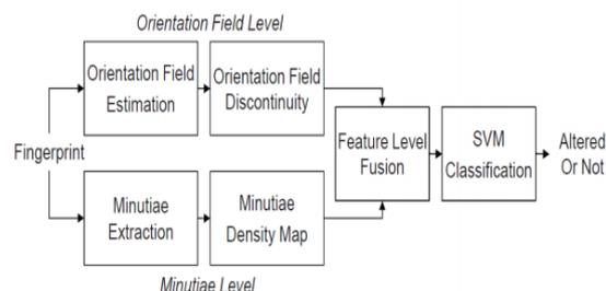
Fig 3. System Architecture
