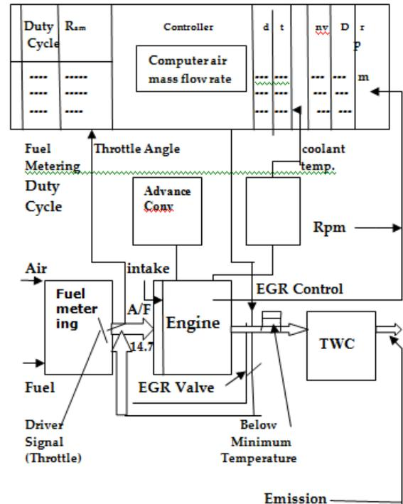
Fig. 3(a) Open Loop Control
