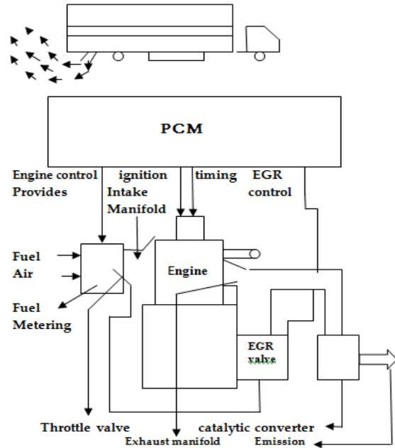
Fig: 4(a) Major Controller out-put to Engine.
