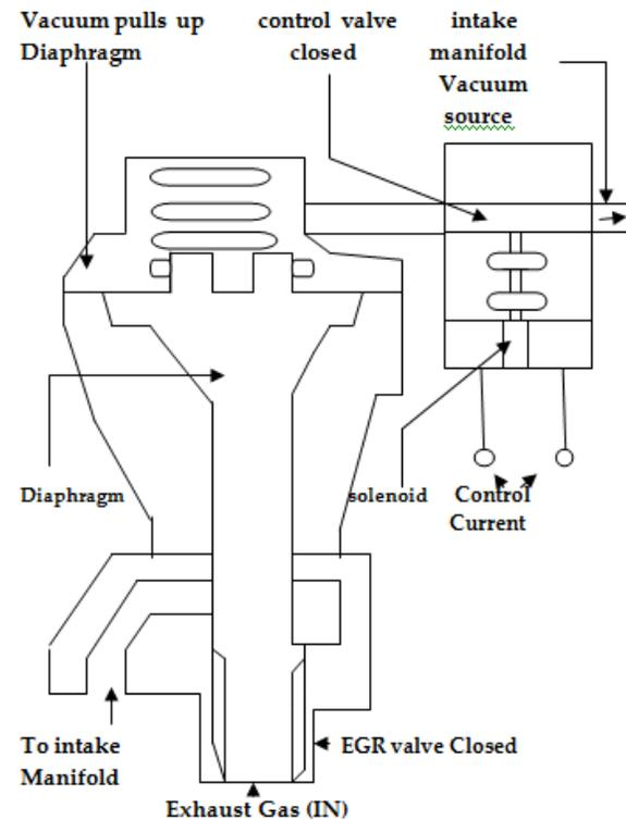
Fig. 6(a) EGR Actuator Control
