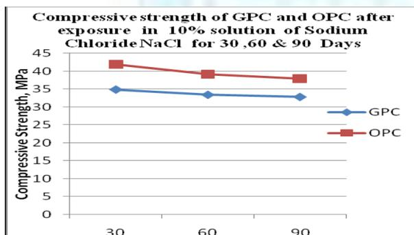
Fig 4: Effect of sulphate and chloride salts
