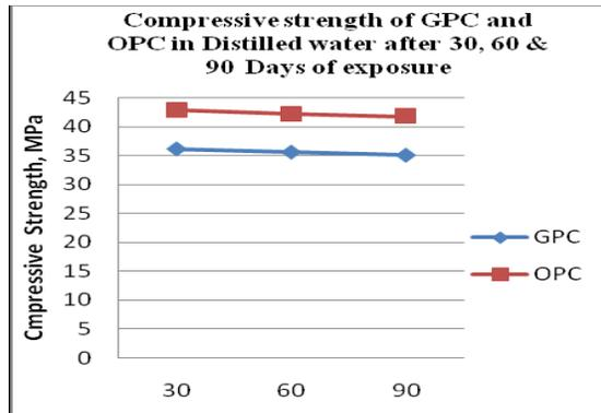
Fig 3: Compressive strength of GPC and OPC in distilled water.
