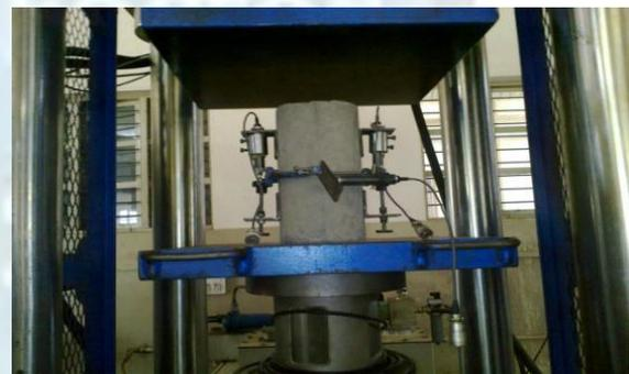
Fig.1 Set up for measuring modulus of elasticity
