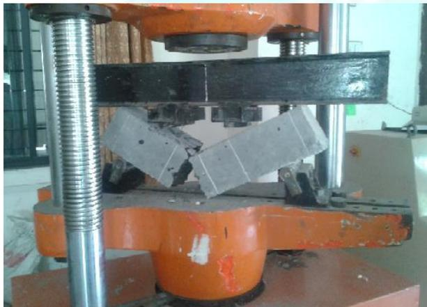
Fig.1: Flexural test setup
