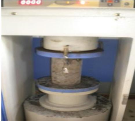
Fig 2: Compression Test on Cube and Cylinders
