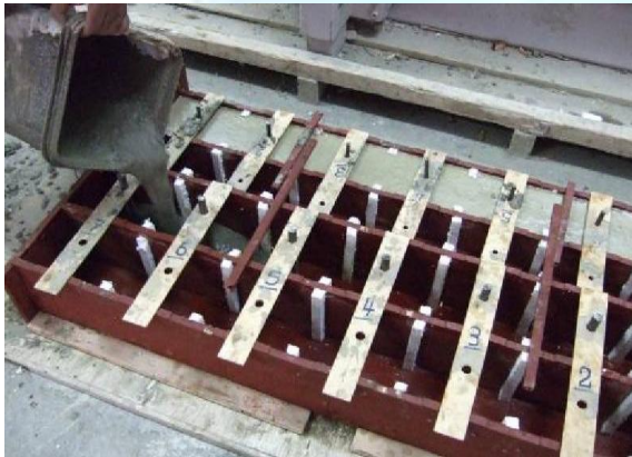
Fig. 1. Preparation and testing of push-out test specimens
