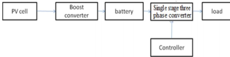
Figure 2: Block Diagram
