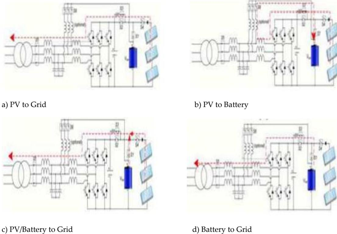
Figure 4: All Operation Methods of RSC
