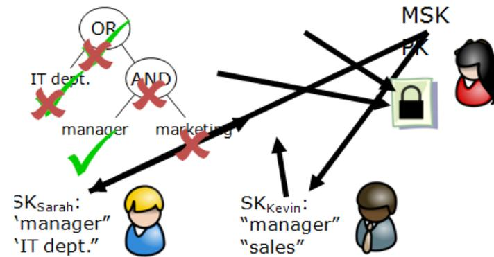
Fig 4. Remove File Storage: Access Control via CP-ABE
