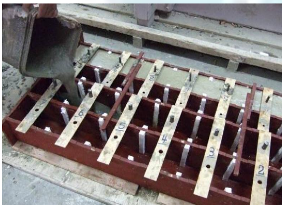
Fig. 1. Preparation and testing of push-out test specimens
