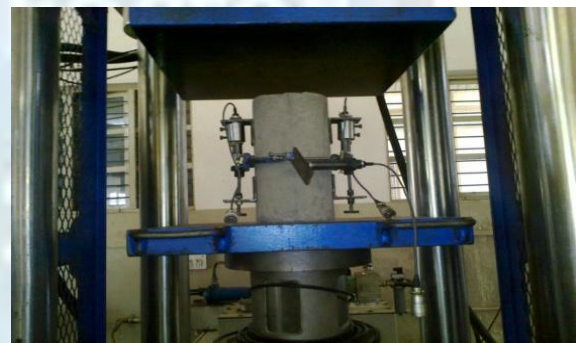
Fig.1 Set up for measuring modulus of elasticity
