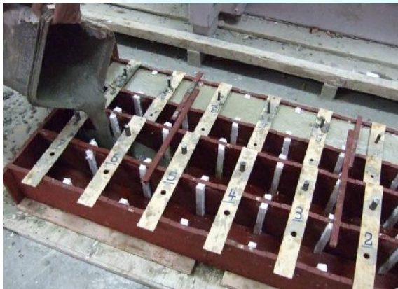
Fig. 1. Preparation and testing of push-out test specimens
