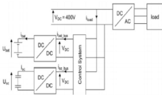
Figure 4: Topology of the controlled SCs/battery Combination
