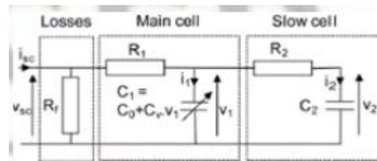
Figure 2: Super-Capacitor simplified circuit: two branches model
