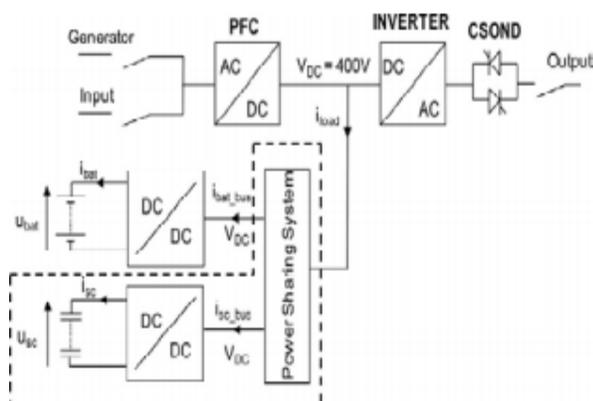
Fig1. Topology of the 500-kVA UPS
